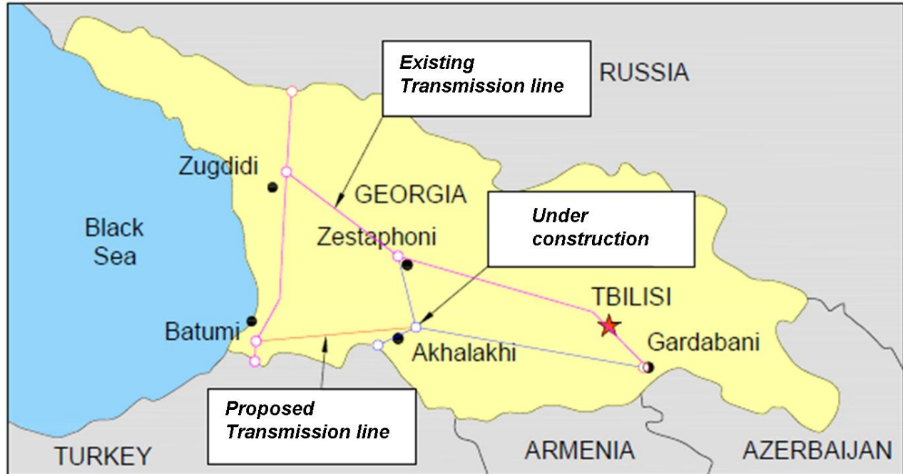
Figure 2.7: Georgian Transmission System Situation Plan
