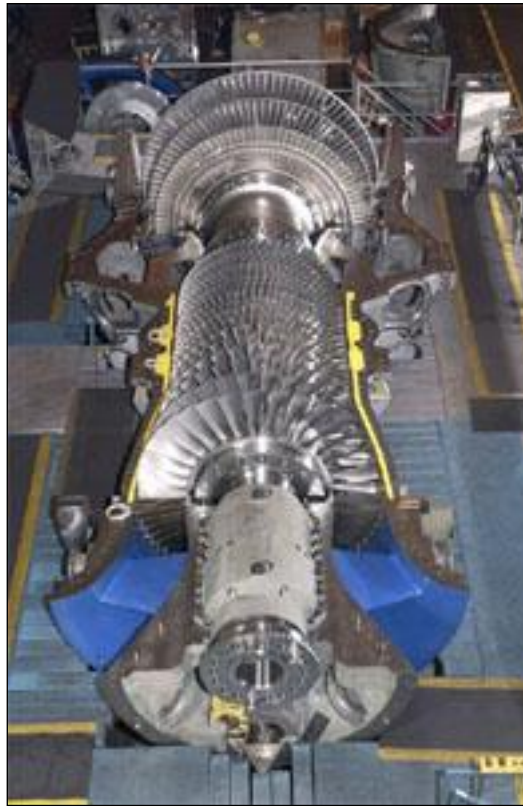
Figure 3-11 9FB Type Gas Turbine
