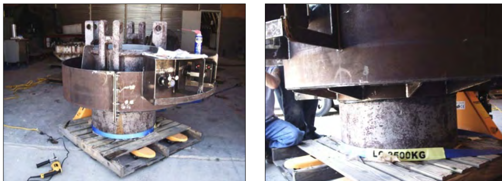
Figure 3-4. Fabrication work on drip pan for slip joints.
