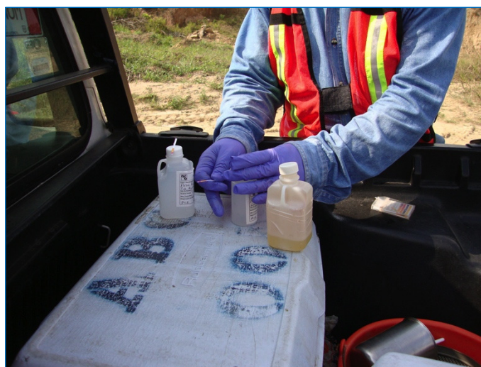
Picture J.3 Ph measurement once the nitric acid had been added
