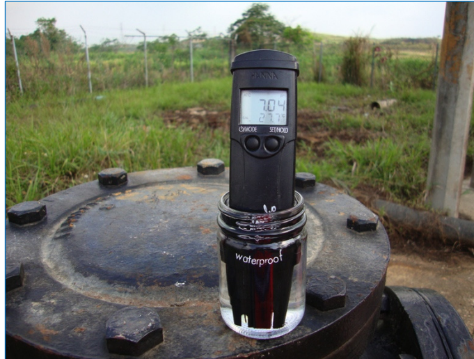
Picture J.J Field measurement of hydrogen potential (pH), EC and temperature
