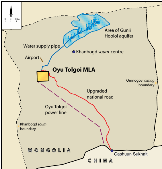
Figure 5: Oyu Tolgoi MLA and other project features including borefield and infrastructure corridor
