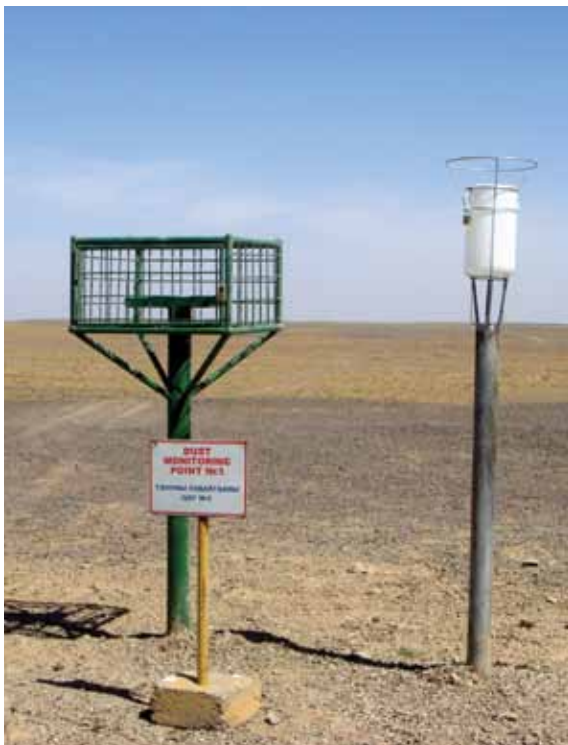
Dust monitoring station in the project area (left) which is subject to frequent dust storms in the spring (right)
