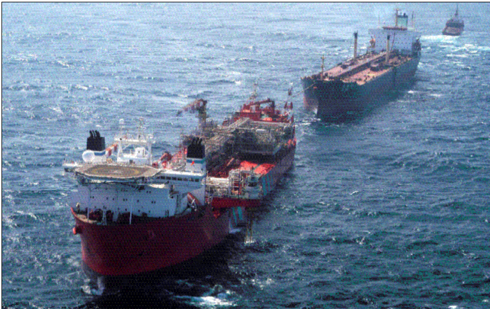
Figure 3.13. Example of tandem offloading between a floating production, storage, and offloading (FPSO) vessel and shuttle tanker (From: Minerals Management Service, 2008).
