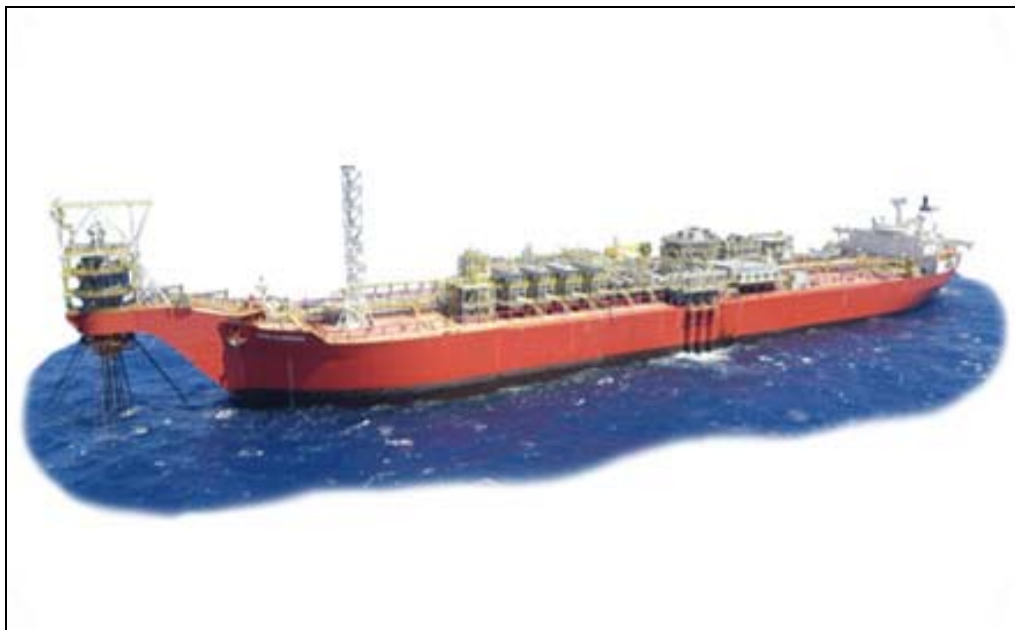
Figure ES.3. Schematic of possible FPSO configuration based on conversion of the very large crude oil carrier (VLCC) Ohdoh .
