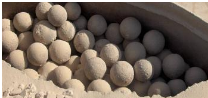
Fig. (1.9): Steel balls used for grinding inside the ball mill
