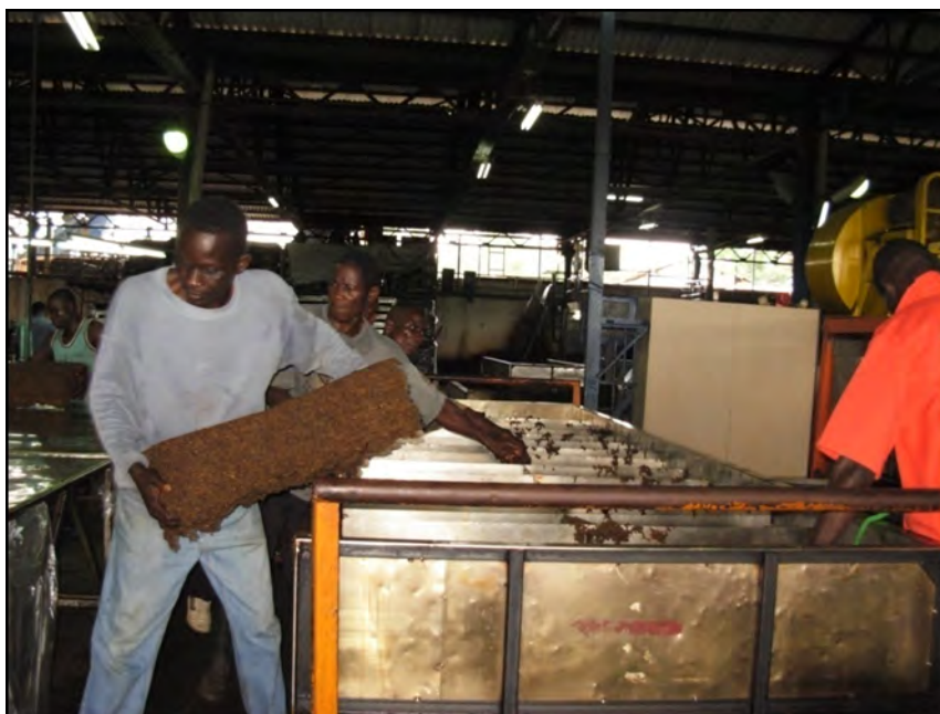
Figure 5-11: Dried rubber biscuits being unloaded from the dryer's trolley. Note the lack of use of safety equipment by workers.
