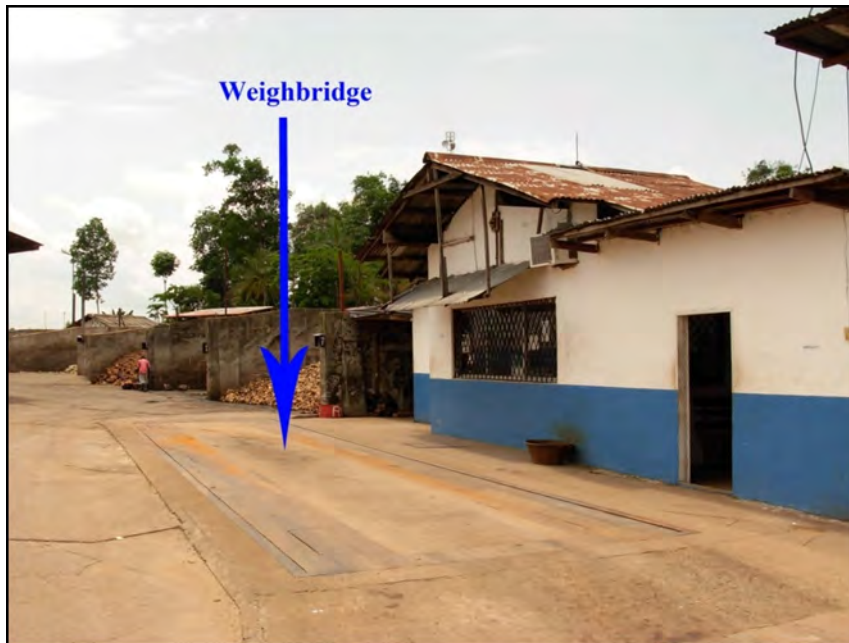
Figure 5-8: SRC's weighbridge located at the factory's site.
