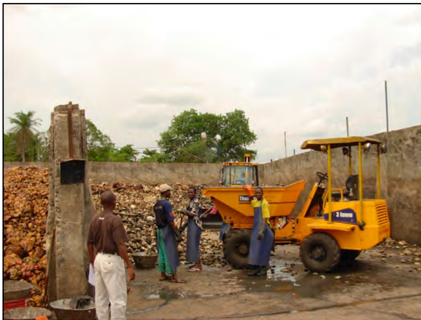
Figure 5-9: Collection of coagulum. Note that basic occupational safety equipment such as masks are not used by the workers.
