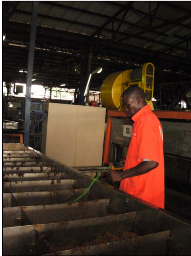
Figure 5-12: Internal temperature of biscuits being measured.
