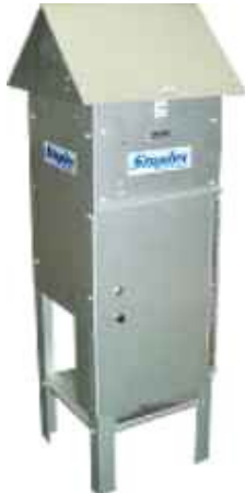
(e): Stationary PM monitoring station
