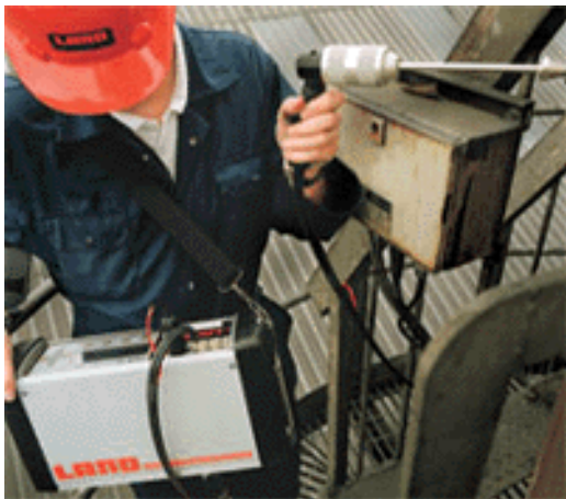
(c): Portable gas analyzer
