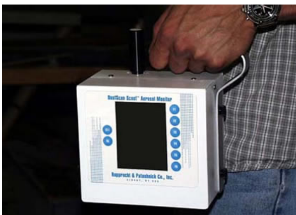
(b): Portable hand-held particle counter
