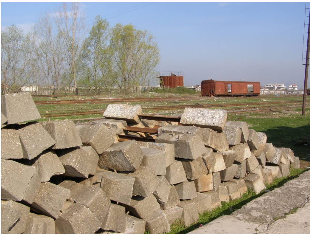
Figure 25 Gjorm Yard – Concrete Bi Block Sleepers
