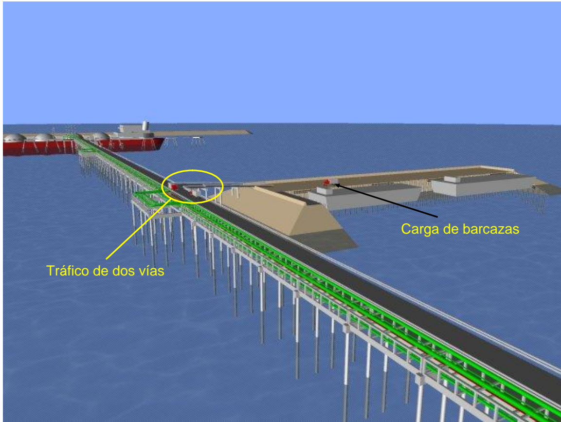
Figure 2.5 Modifications to the Trestle
