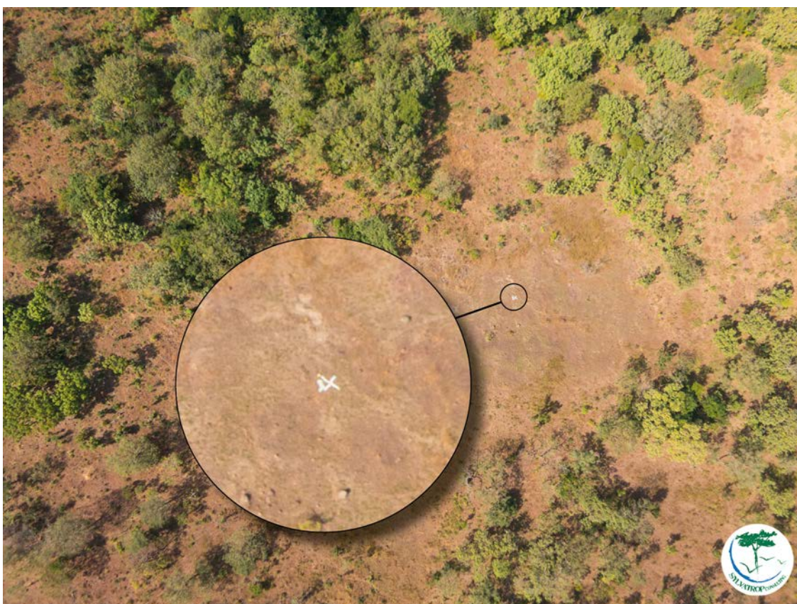
Figure 6 : Example of one Ground Control Point pictured by the drone
