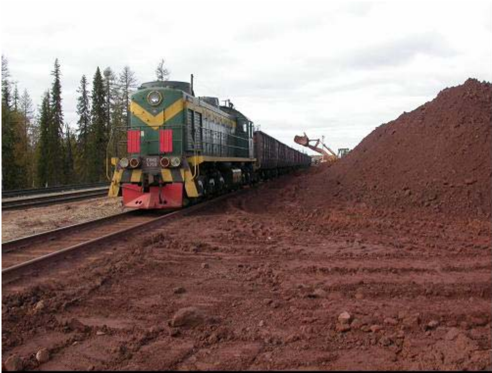
Plate 6: Central Blending Yard (CBY) and rail loading facility where high concentrations of fines are generated
