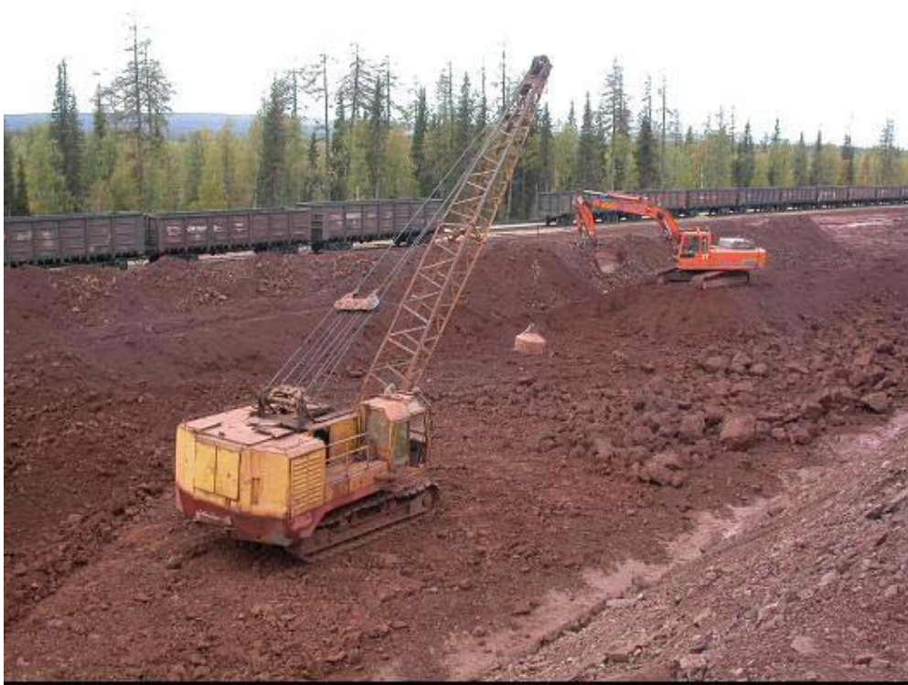
Plate 3: Crushing the oversize bauxite using a dragline with a wedge which is hoisted and dropped on the oversize bauxite. Note the crushed material around the drag line, with the oversize material ahead of the dragline.
