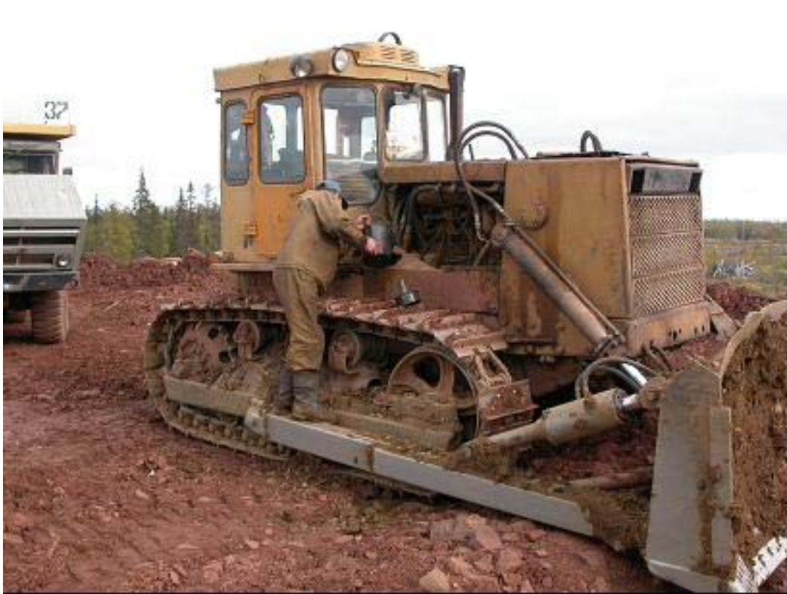
Plate 22: The same bulldozer operator refilling the crankcase of the bulldozer
