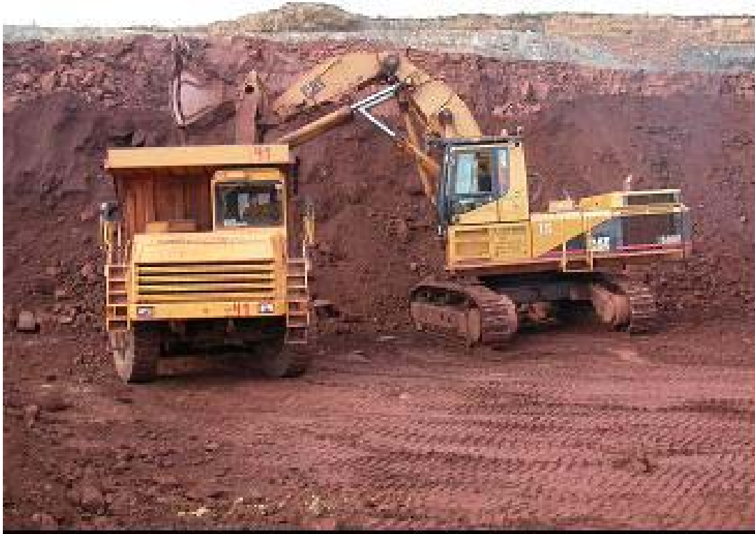
Plate 2: An excavator loading bauxite on to a 30 tonne truck for transport to the Central Blending Yard. Note also the layer of basalt above the bauxite and the overburden and top soil layers above that.
