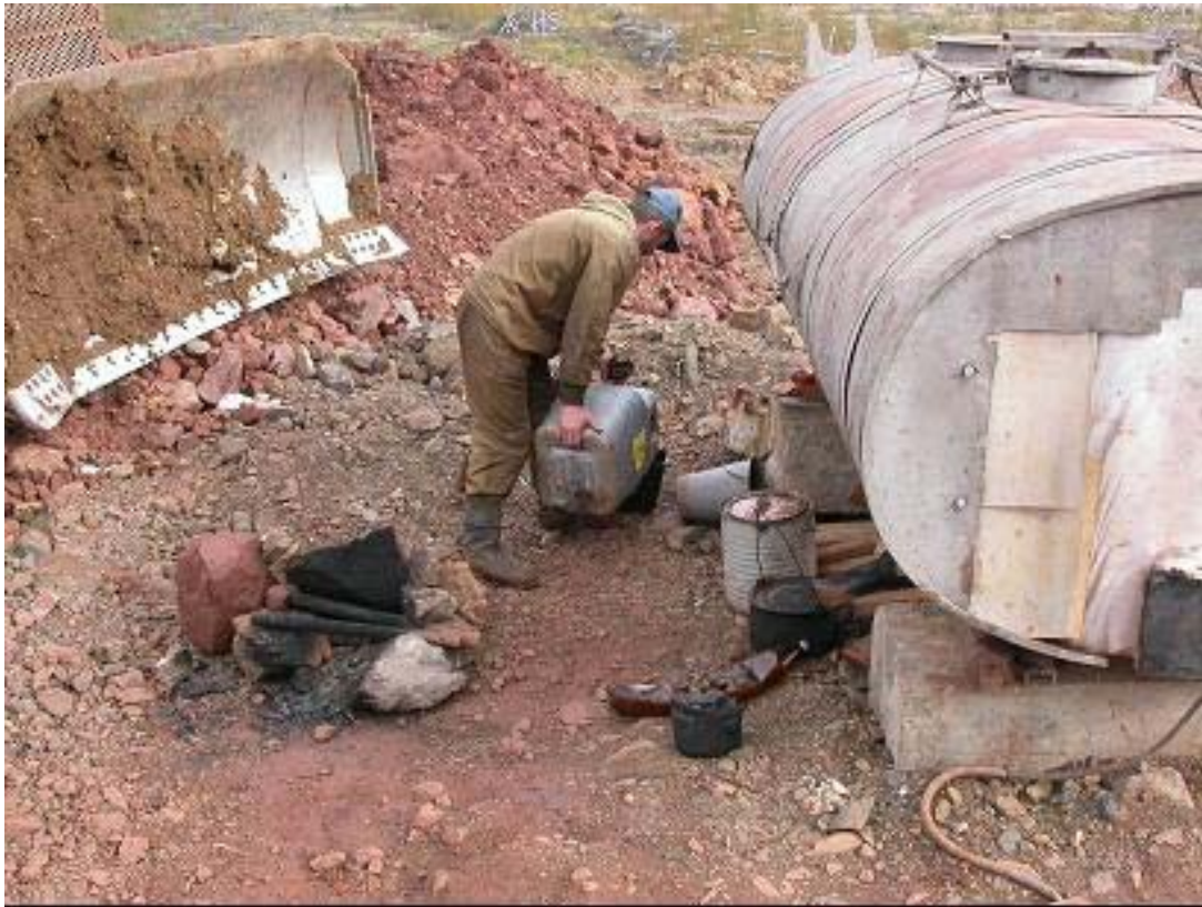
Plate 21: An example of the ad hoc vehicle and plant maintenance seen at the mine. The operator is filling a can with oil to top up the crankcase on a bulldozer. Note the cooking fire and pots in the foreground.
